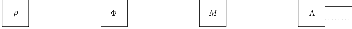
Figure 4: Pictorial representation of quantum devices. From left to right: a quantum state (preparator), a quantum channel, a measurement, and an instrument. Diagrams are to be read from left to right. Quantum systems are depicted by solid lines, while classical systems are represented by dotted lines.
