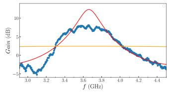
FIG. 6. The measured gain of the TWPA (blue line) for the pump frequency of 3.38 GHz. Orange and red curves are the results of the standard CME and the model with reflections for  $\Gamma_p = 0.72$ , respectively.
