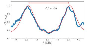
FIG. 5. (a) Calibrated weak signal transmission without pumping tone (blue line). Fit of the data by Fabry-Pérot oscillating transmission (9) (red curve). The parameters of the fit;  $\Gamma_s$  and v, are listed in Table II.
