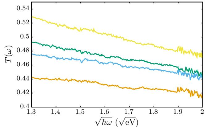
FIG. 2. Frequency dependence of transmission through MoC thin films on sapphire substrates for the same set of films and with the same color coding as in Fig. 1.
