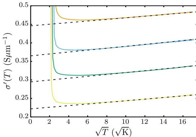
FIG. 1. Temperature dependence of dc conductivity for a series of 5-nm-thick MoC films. The sheet resistance of the films at room temperature is (from bottom to top)  $R_{\square} = 720, 590, 500,$  and  $415 \Omega$ . Fits to Eq. (3) are shown as well.
