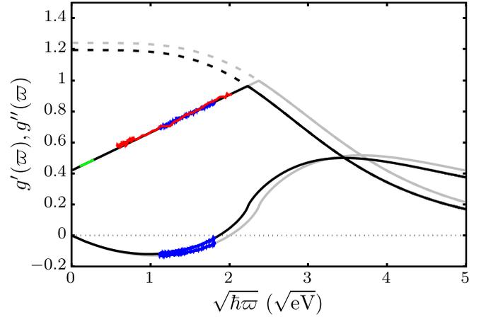
FIG. 4. Results of the prolongation procedure described in the text for  $\epsilon_{\infty} = 1$  (gray lines) and  $\epsilon_{\infty} = 1.4$  (black lines), applied to the data from Fig. 3 (with the same color coding). The dashed lines denote the continuation of the high-frequency behavior (i.e., conductance in the absence of quantum corrections) to low frequencies.
