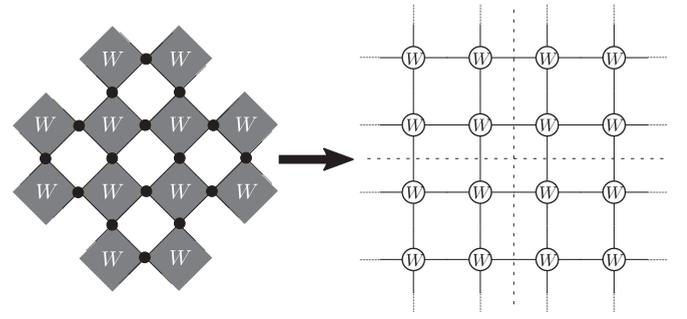
FIG. 2. Icosahedron model on the diagonal lattice, where  $W$  on each black plaquette represents the local Boltzmann weight of Eq. (2). The partition function can be represented by a tensor network on the square lattice. The dashed lines show the division of the system into quadrants corresponding to CTMs.
