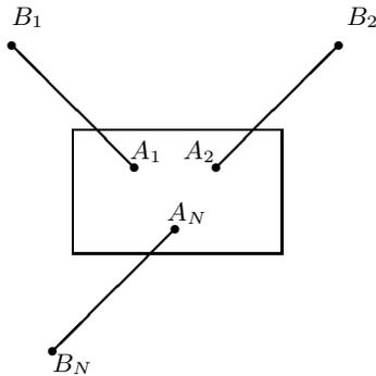
FIG. 7:  $N$  Werner states are distributed between  $A_i$  and  $B_i$  (for  $i = 1, 2, \dots, N$ ) and a GHZ basis measurement is performed at  $A_1, A_2, \dots, A_N$ .
