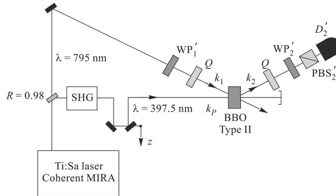
Fig. 2. Schematic description of the experimental verification of the universality of the flip operation
