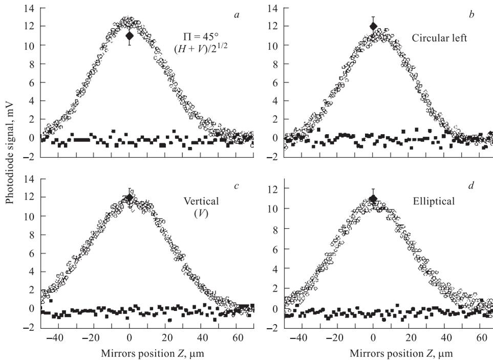
Fig. 3. Experimental verification of the universality of OPA
